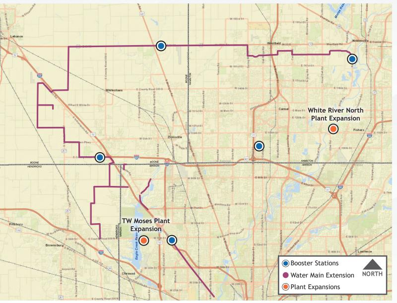
To increase its treatment capacity to nearly 300 MGD, Citizens will expand two surface water treatment plants, extend water mains to connect with the City of Lebanon, upgrade several booster stations, and add water storage tanks.
